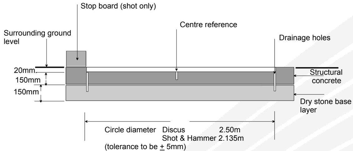
**Figure 7 Cross-section of throwing circle construction**
