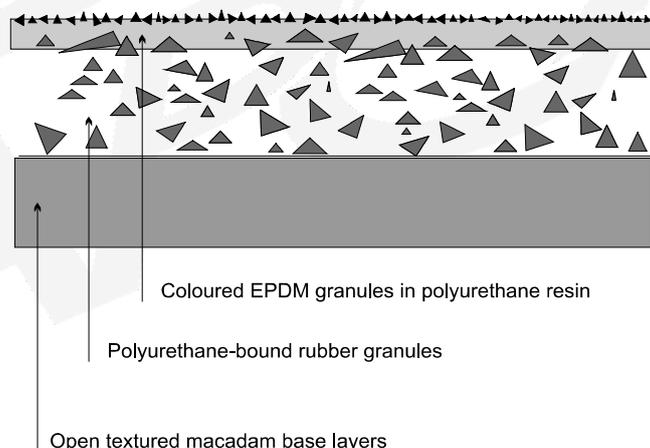
**Figure 15 Diagrammatic cross-section of sandwich system**
