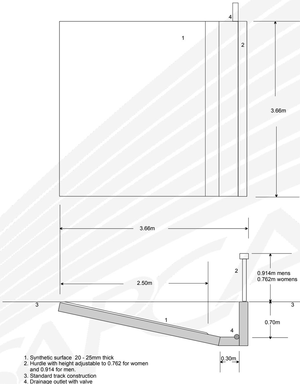
**Figure 5 Plan and cross-section of water jump**
