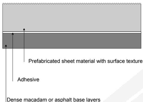
**Figure 17 Diagrammatic cross-section of a prefabricated system**
