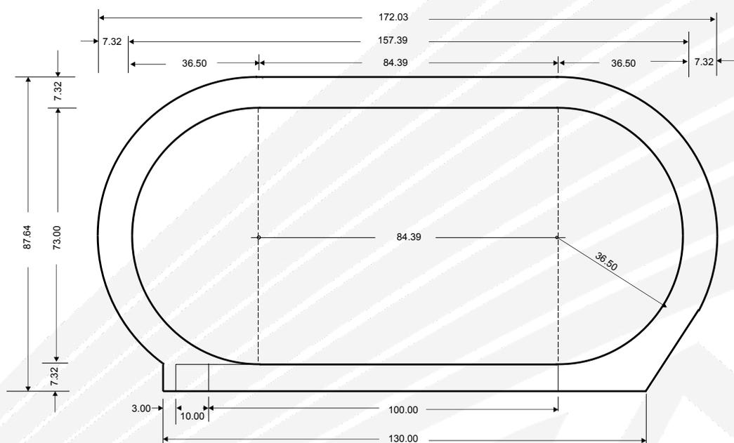
possible, a new six-lane track will be constructed to the standard dimensions in Fig 1.
