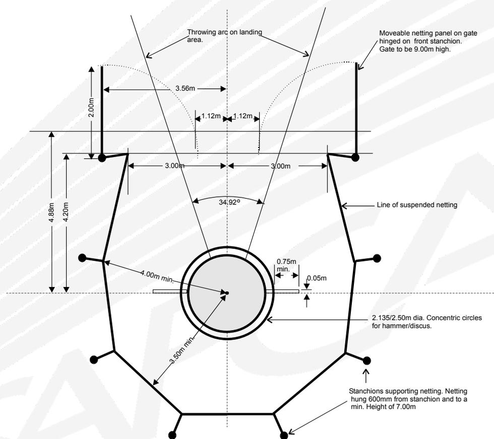
Figure 9 Cage for hammer or discus using concentric circles
