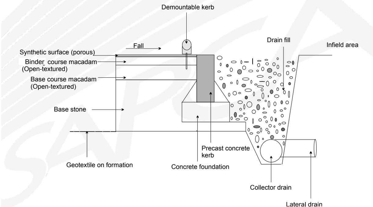
**Figure 12 Typical cross-section of track (porous and sandwich systems)**
