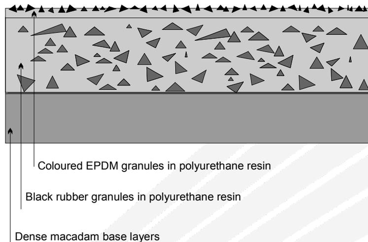
**Figure 14 Diagrammatic cross-section of solid system**
