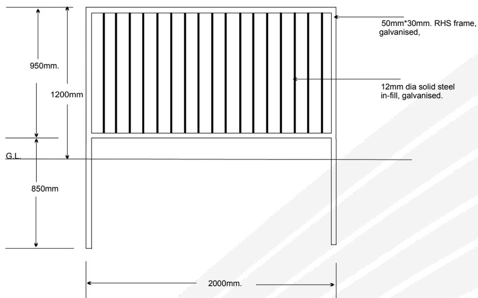
Figure 18 Pedestrian barrier detail
