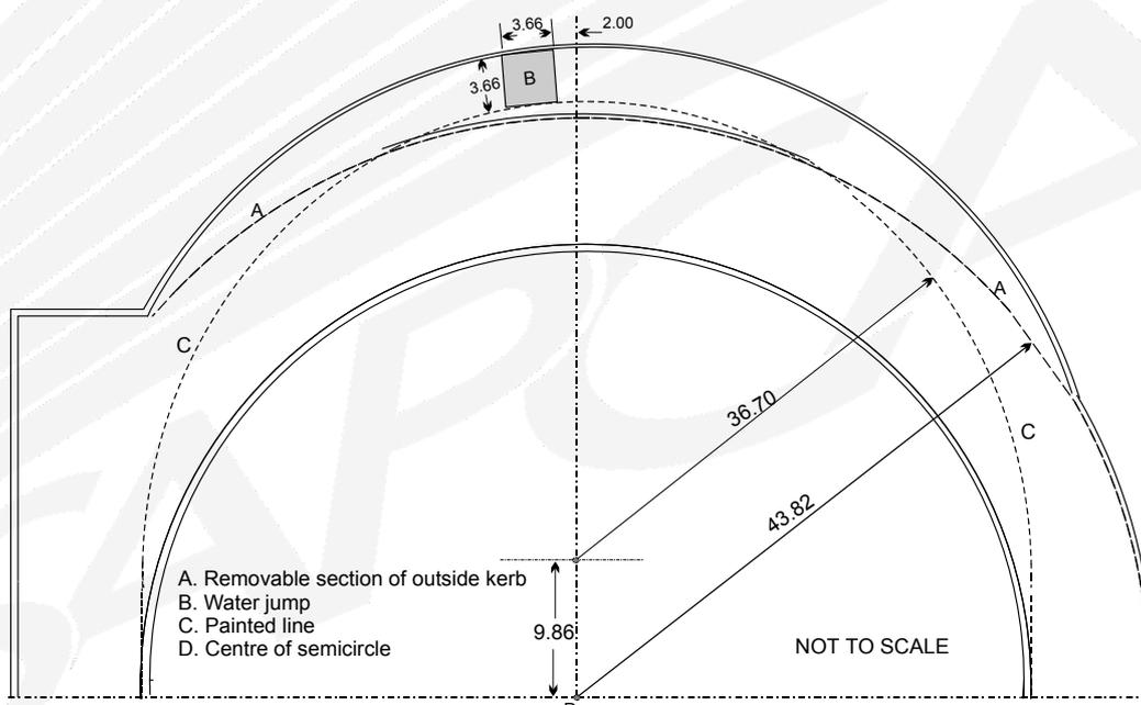
Figure 4 Steeplechase widening on outside of bend of six-lane track
