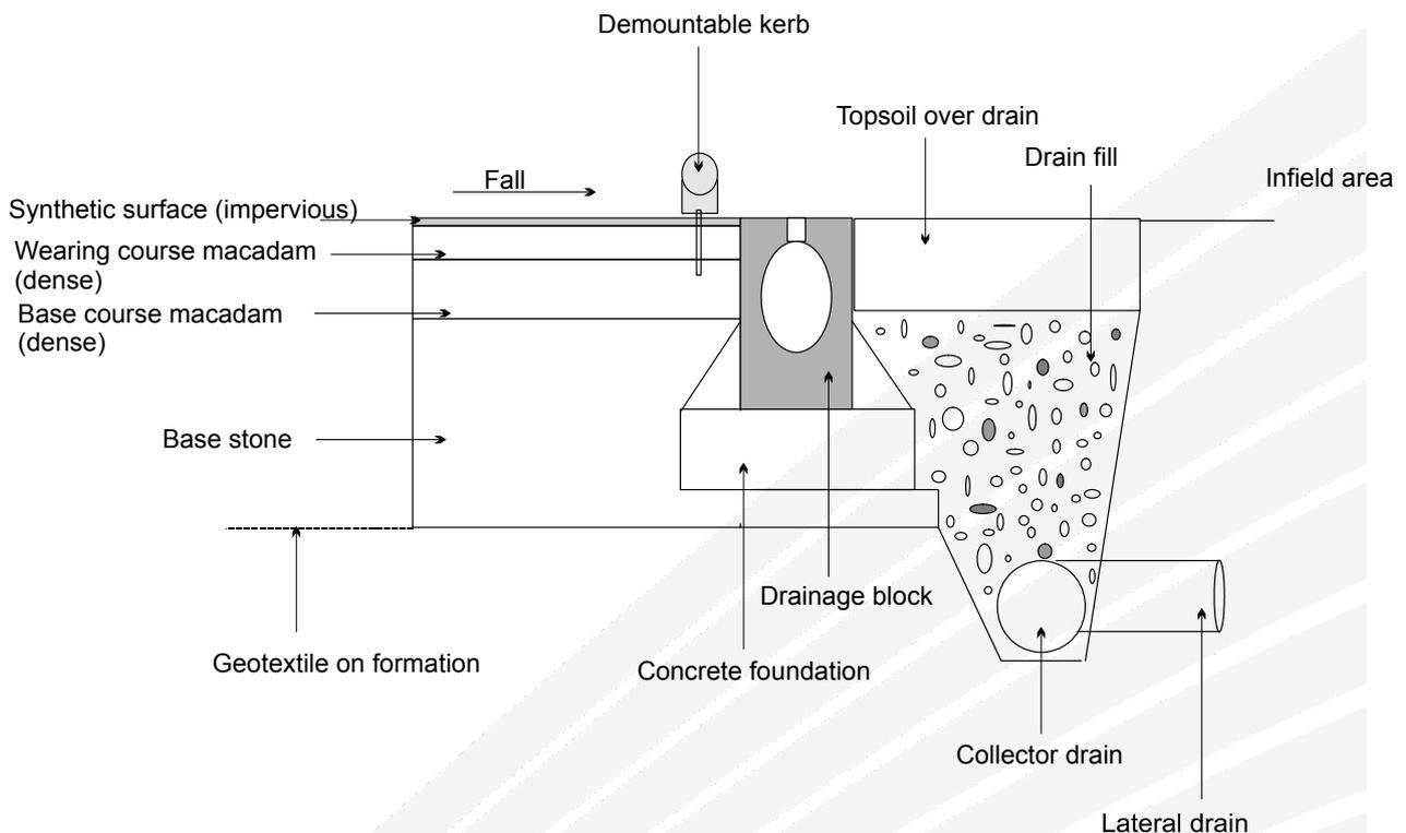
**Figure 13 Typical cross-section of track (solid system)**
