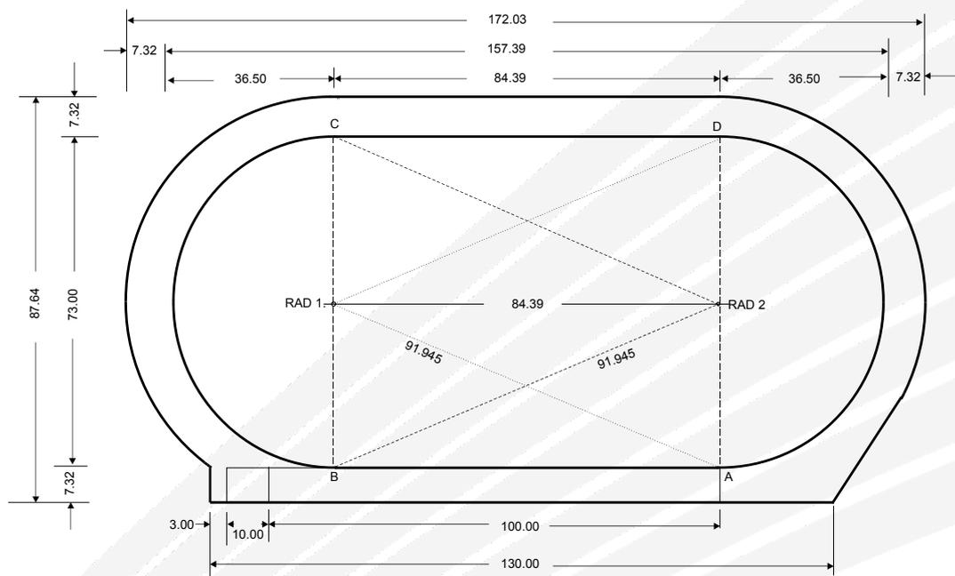
**Figure. 2 Setting-out dimensions of a standard 400-metre, six-lane track**
