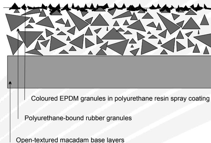
**Figure 16 Diagrammatic cross-section of porous system**
