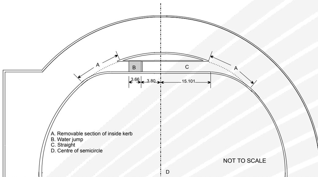
Figure 3 Steeplechase widening on inside of bend of six-lane track
